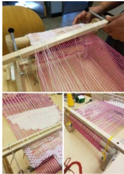
Figure 6. (top) Developing new methods for maximizing the usable lengths that could be reharvested from woven fabrics required us to modify weaving equipment. These process pictures show how we inserted an extra beam into the loom to hold a modified warp (on top of the more traditional and existing loom warp). (bottom) The additional warp structure is created by adding additional beams secured in front and back for shape weaving with continuous warp.
