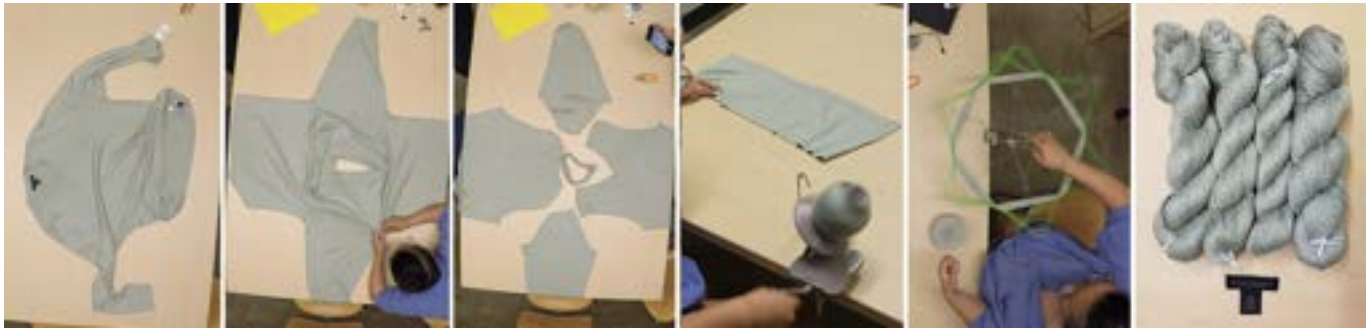
Figure 2. The process of unravelling a knit garment and reclaiming its yarn. a) The initial garment. b) Separating the first set of seams. c) The garment pieces fully separated. d) Unravelling each piece with the help of a yarn winder. e) Winding the unravelled yarn into loops to prevent tangles. f) The reclaimed yarn shown, after washing, with the original garment label.
