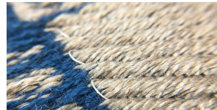
details of the conductive yarns peaking to the surface at the edges of the pocket
